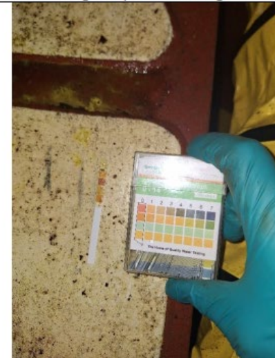
pH paper test – result pH 0
